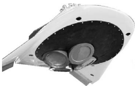
Fig. 1. Endeco/YSI type 850 V-Fin with 75 kHz RDI Long Ranger ADCP. The V-Fin is approximately 1.3 x 1.4 x 0.7 meters.
