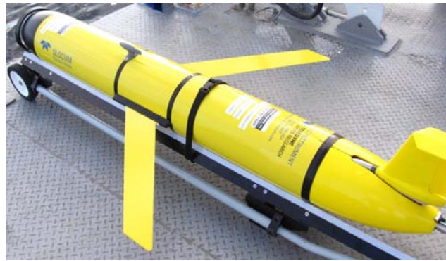
Figure 1. Teledyne-Webb Research Slocum 1000 m autonomous glider.
